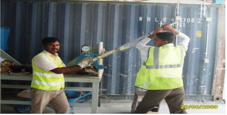
Matin Manman is performing the necessary testing for the "Calibrated wrench Method" for different bolt sizes. (20/06/2009)
